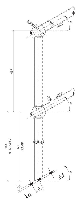
'a' ANGLE DRILLINGS ANGLE STANCHIONS CAN BE MADE TO ORDER WITH ANY ANGLE DESIGNATED BETWEEN 1° ~ 45°
